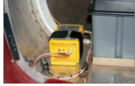
Just looking at this Artex ME406 makes the install look trivial. The hidden cost is in wiring to the remote switch and optional GPS connection.
