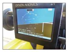
In a taildragger like the J-3, the D1's horizon line, right, has to be adjusted to account for the tail-low ramp position. That's done with the small rocker switch on the right side of the bezel, lower photo. Roll errors can also be cancelled with the same control. The D1's internal battery has a four-hour endurance, but it also has a ship's power option.
