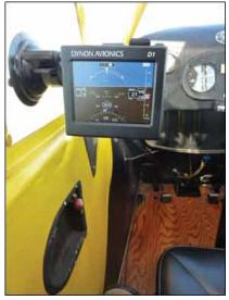
Dynon's D1 has a genuine MEMS solid-state gyro system for pitch and roll indications. Since it has no air data access, speed and altitude are GPS derived through a built-in receiver. Similarly, the heading indicator is also GPS ground track, not magnetic heading. The D1 has a remote antenna, but doesn't seem to need it.
