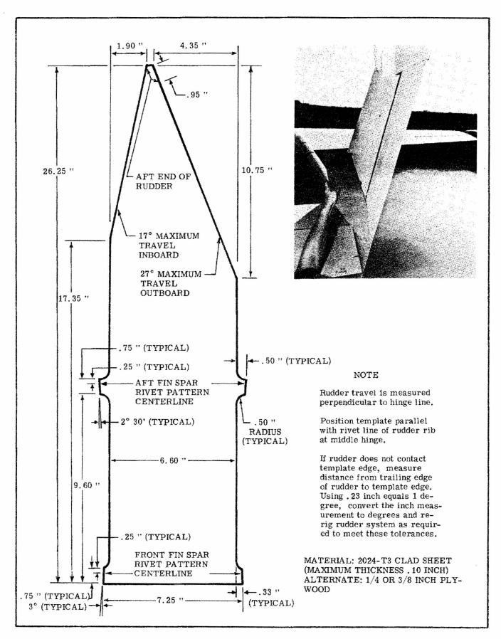
Figure 9-4. Measuring Rudder Travel
