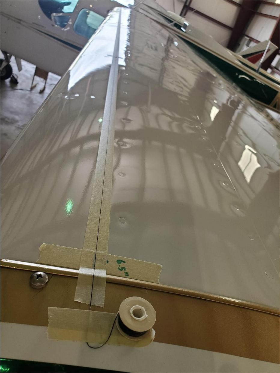
Templates are peel and stick contact paper with mild adhesive backs. Installation manual is clear and easy to understand on placement.
