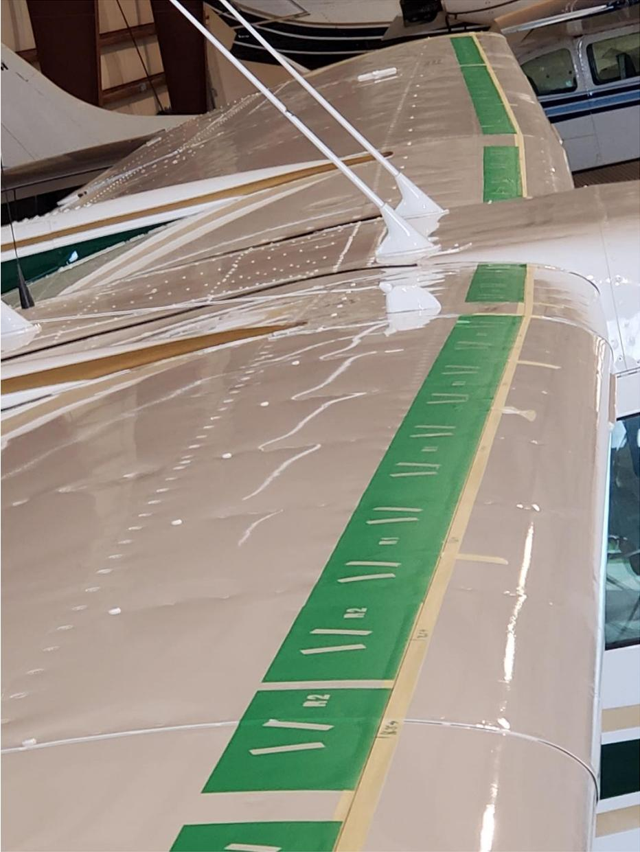
And the first ones go on. Pretty good color match! I followed the instructions about clean up right away so have very little glue residue—glue goes on clear but dries brown, so wiping away excess with alcohol-soaked Q-tips (provided in kit) helps ensure very little glue residue is visible. Process I used was double check template position, glue on all VGs for that template, then do the next, then return to the previous and remove template and wipe away excess glue.
