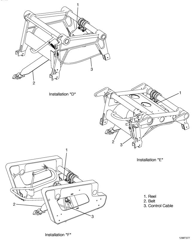
Figure 1. Identification of Secondary Seat Stop Installation Configurations (Sheet 2)
