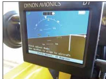
In a taildragger like the J-3, the D1's horizon line, right, has to be adjusted to account for the tail-low ramp position. That's done with the small rocker switch on the right side of the bezel, lower photo. Roll errors can also be cancelled with the same control. The D1's internal battery has a four-hour endurance, but it also has a ship's power option.
