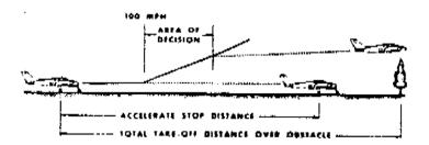
Fig. 5 - Single engine take-off - conventional twin
