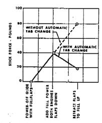
Fig. 3 - Longitudinal trim changes in balked landing goaround
