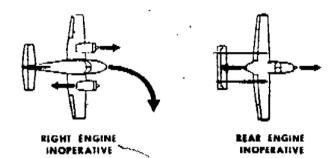
Fig. 4 - Effect of engine failure on directional control
