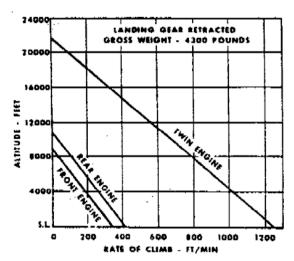
Fig. 11 - Rate of climb versus altitude
