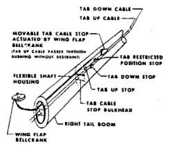
Fig. 2 - Elevator trim/wing flap interconnect system
